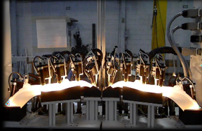
Infra Stake Welding
